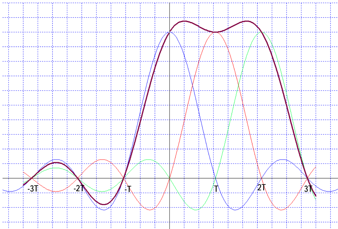
Figure 16: The actual signal on the wire is the sum of the individual pulses. Here, the heavy trace indicates the actual signal.
